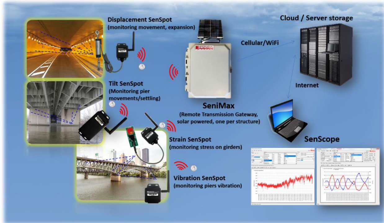
Illustration of Resensys SHM based on SenSpot sensors for fracture critical monitoring
