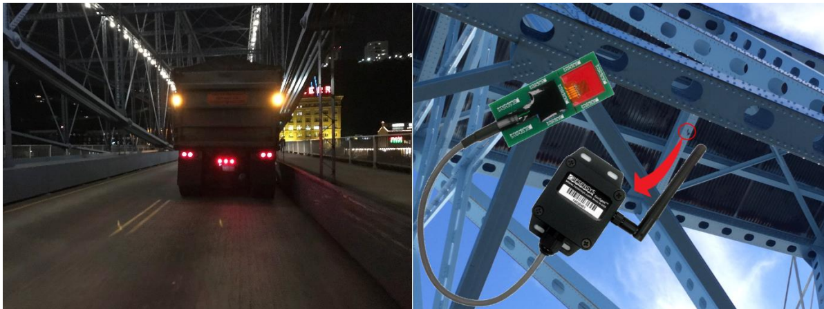
SenSpot™ as test tool for bridge load rating by using truck(s) tests
