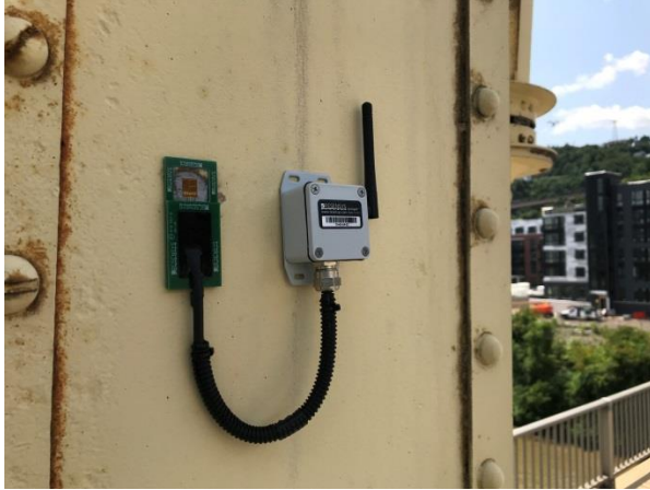
Resensys Wireless Strain SenSpot™ sensor installed on the bridge for bridge load rating
