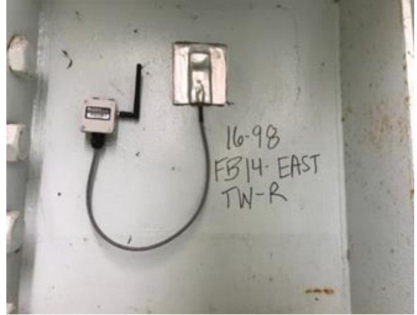
Resensys Wireless Strain SenSpot™ sensor installed on the bridge for bridge load rating
