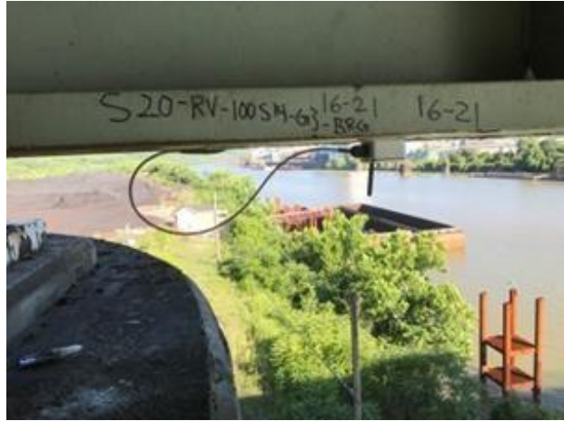
Resensys Wireless Strain Gauge SenSpot™ sensor installed on the bridge for fatigue analysis using the rainflow methodology
