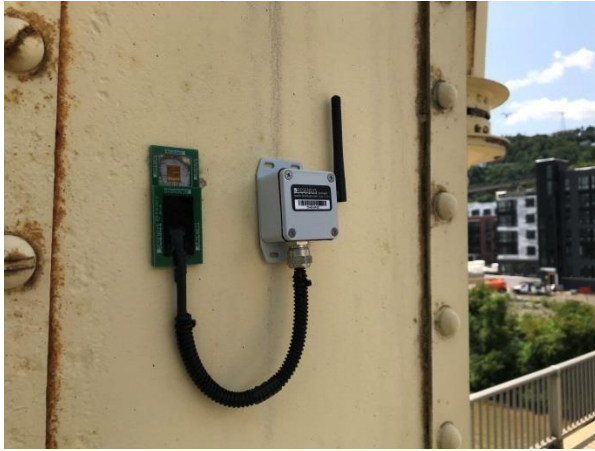
Resensys Wireless Strain Gauge SenSpot™ sensor installed on the bridge for fatigue analysis using the rainflow methodology
