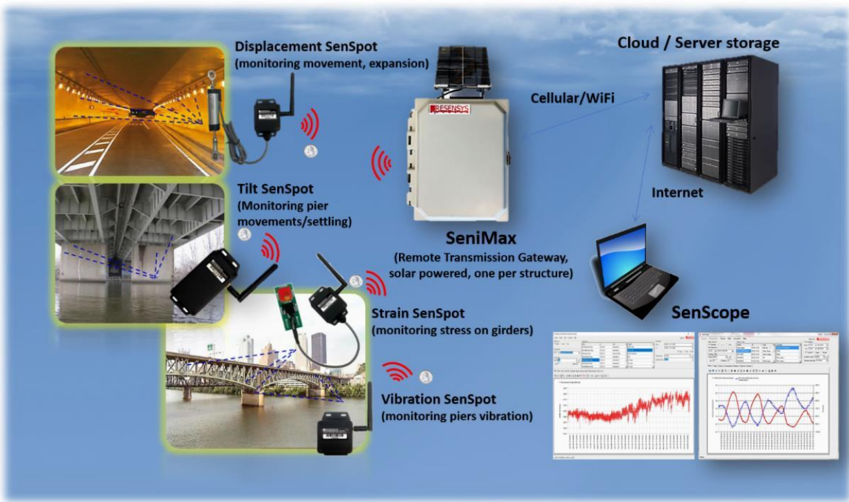
Illustration of Resensys SHM based on SenSpot™ sensors for remote monitoring bridges under extreme load of permit loads
