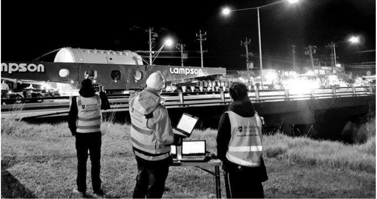
Remote monitoring Australia concrete bridges under extreme loads: Resensys wireless monitoring
