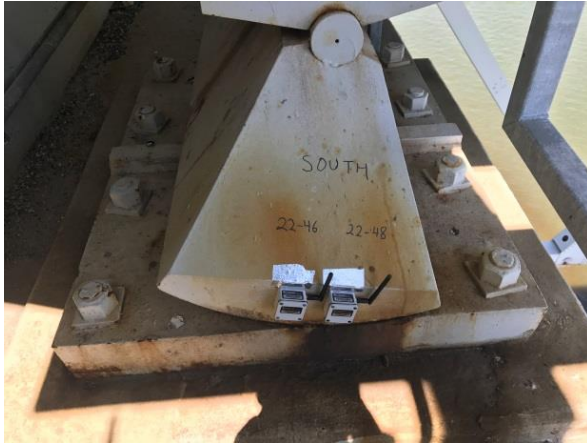
Resensys Wireless Tilt/ Inclination SenSpot sensors on bridge bearings to assess bearings functionality
