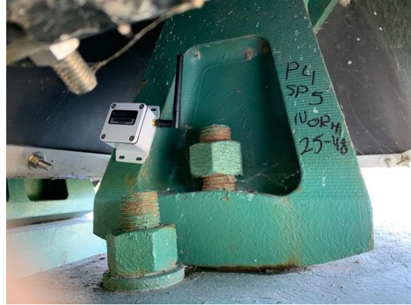
Resensys Wireless Tilt/ Inclination SenSpot sensors on a bridge bearing to assess bearings functionality
