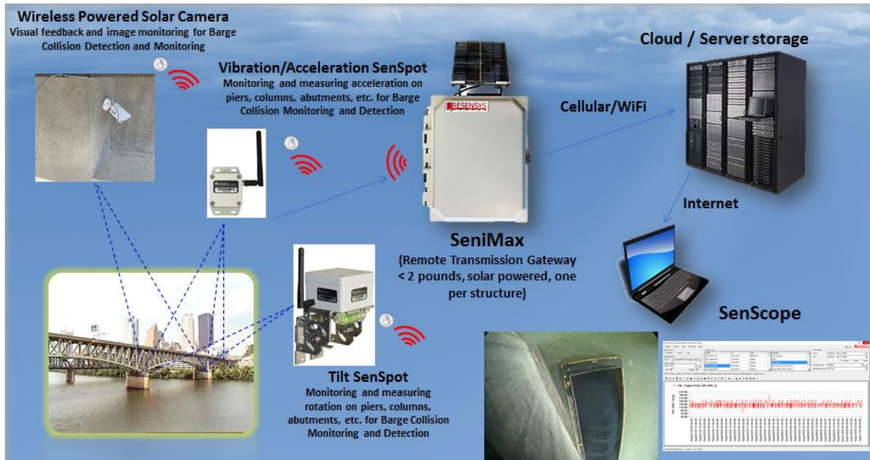
Illustration of Resensys SHM based on SenSpot™ sensors and Wireless Solar Powered Camera for barge collision detection and monitoring of bridge piers
