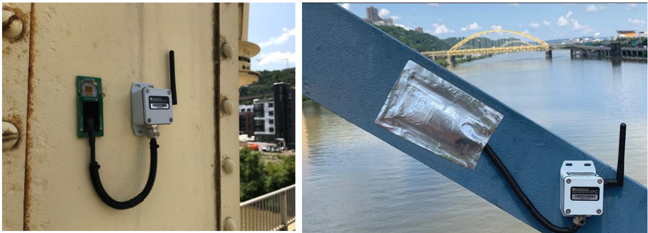
Resensys Wireless Strain SenSpot™ sensor installed on the bridge for bridge routine load rating
