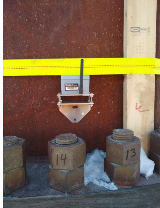
Monitoring potential inclination shaft or base of the turbine at outside surface of the turbine. Wireless High-Resolution Tilt (HRT) SenSpot™s can be installed outside surface of the turbine base at multiple locations.
