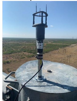
Wireless 2D/3D Anemometer SenSpot™ at a turbine for monitoring wind and environmental condition
