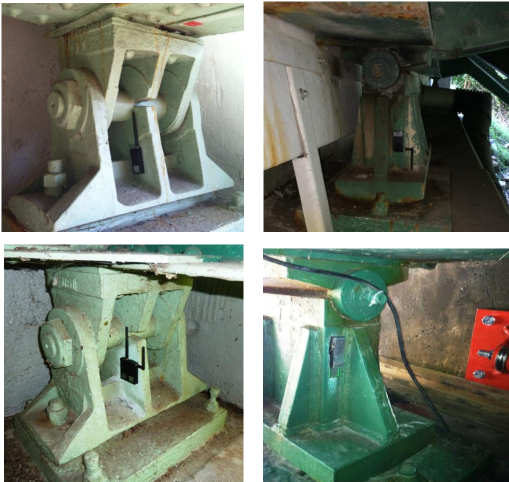
Figure 2: Some deployed tilt SenSpots on the rocker bearings.
