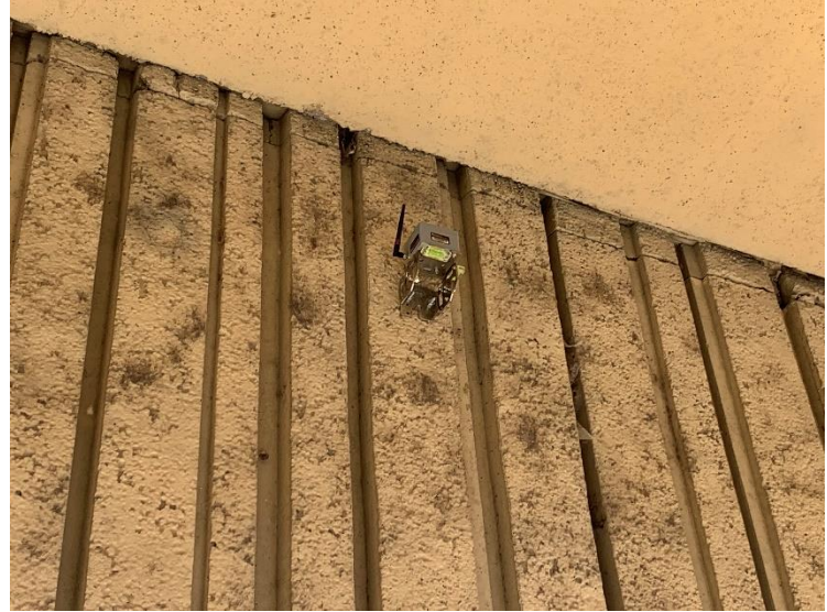
Resensys Wireless Tilt SenSpot™ sensor for measuring and monitoring tilt/inclination (in two directions) and temperature on the face of a Retaining Wall
