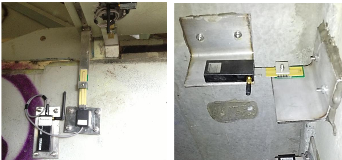
Figure 2: SenSpots used for measuring displacement.
