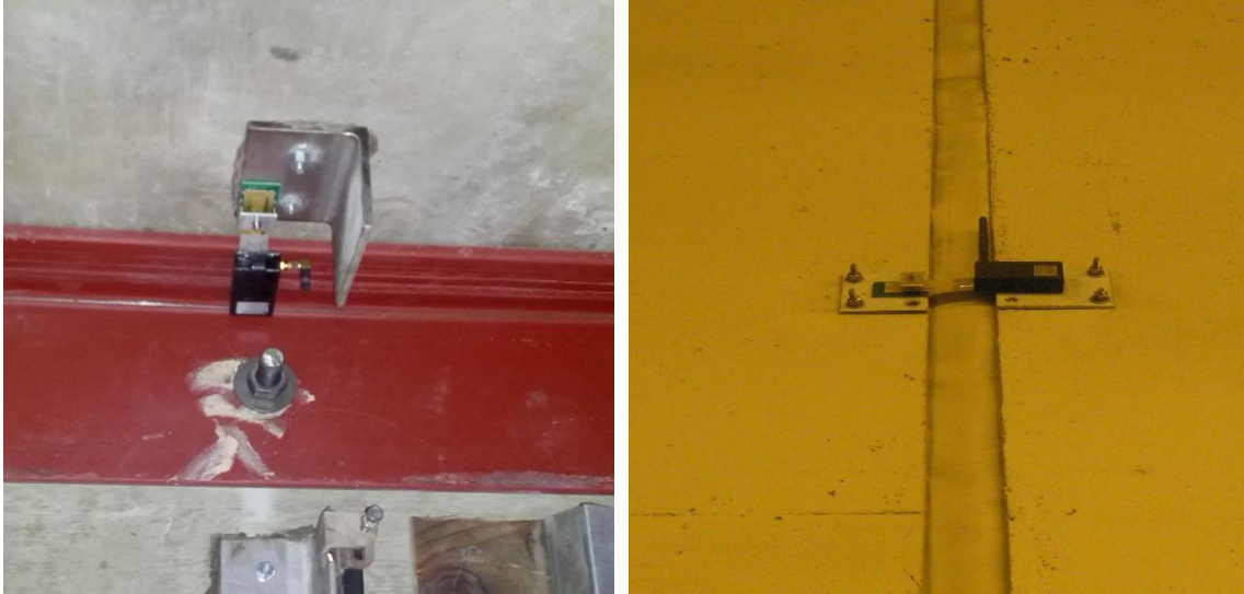
Figure 3: SenSpots used for measuring displacement.
